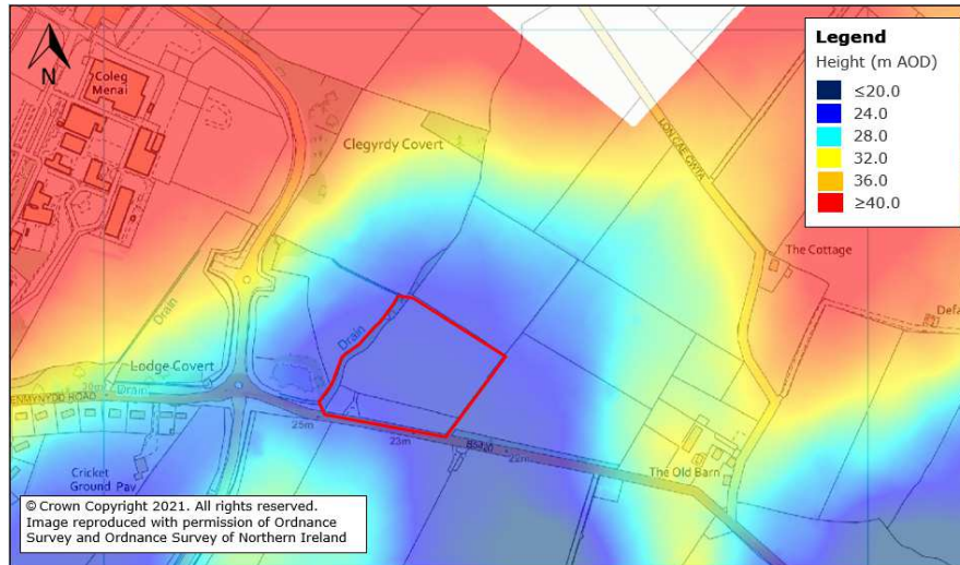
Figure 2: Digital Terrain Model from LiDAR Data
